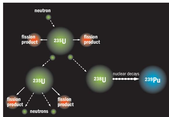
**Figure A.1: A chain reaction produces steady power when the neutrons produced in every fission event produce exactly one further fission event. Plutonium is produced via neutrons that do not produce fission events.**
