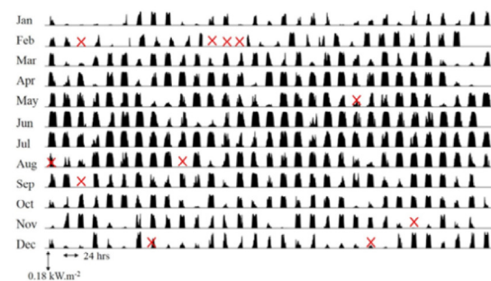
Figure A.6: Power production profiles for tracking panels in Princeton University's 5.4 megawatt solar installation for each day in 2014. Each month's peak hourly output is rescaled to be 180 watts per square meter of panel area. Red crosses indicate days when data are missing for at least part of the day.
