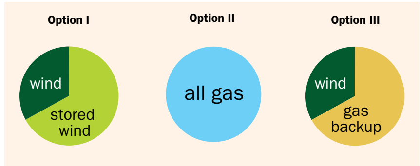
Figure 3.1 Three options for providing one unit of constant power over a full day. Wind is assumed to be available only for the first eight hours. In Option I, three units of wind are collected and two are stored to provide power during the other 16 hours. In Option II, natural gas provides power at a constant rate throughout the day. In Option III, wind provides power during the first eight hours and gas provides the “backup” power during the other 16 hours.
