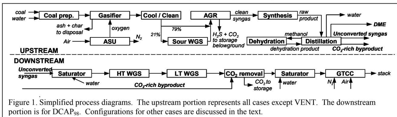
Figure 1. Simplified process diagrams. The upstream portion represents all cases except VENT. The downstream portion is for DCAP<sub>98</sub>. Configurations for other cases are discussed in the text.
