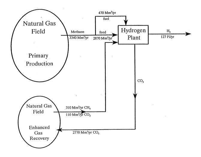
Figure 1. Wellhead Production of Hydrogen from Natural Gas with Injection of the Separated CO<sub>2</sub> into a Depleted Natural Gas Field and Enhanced Natural Gas Recovery as a Result of Reservoir Repressurization.
