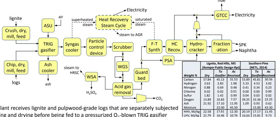
The plant receives lignite and pulpwood-grade logs that are separately subjected to sizing and drying before being fed to a pressurized O<sub>2</sub>-blown TRIG gasifier
