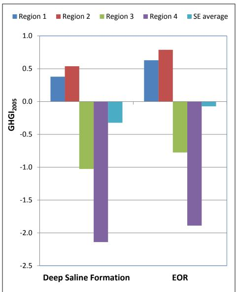
In the medium scenario, with  $CO_2$  stored underground via enhanced oil recovery, lifecycle emissions for combined liquid fuels and electricity supply by LBJ are reduced by about 20% (GHGI<sub>2005</sub> = 0.78) in Region 2, which includes AL and MS. For the weighted-average biomass supply situation in the Southeast, lifecycle emissions are essentially zero (GHGI<sub>2005</sub> = - 0.07).
