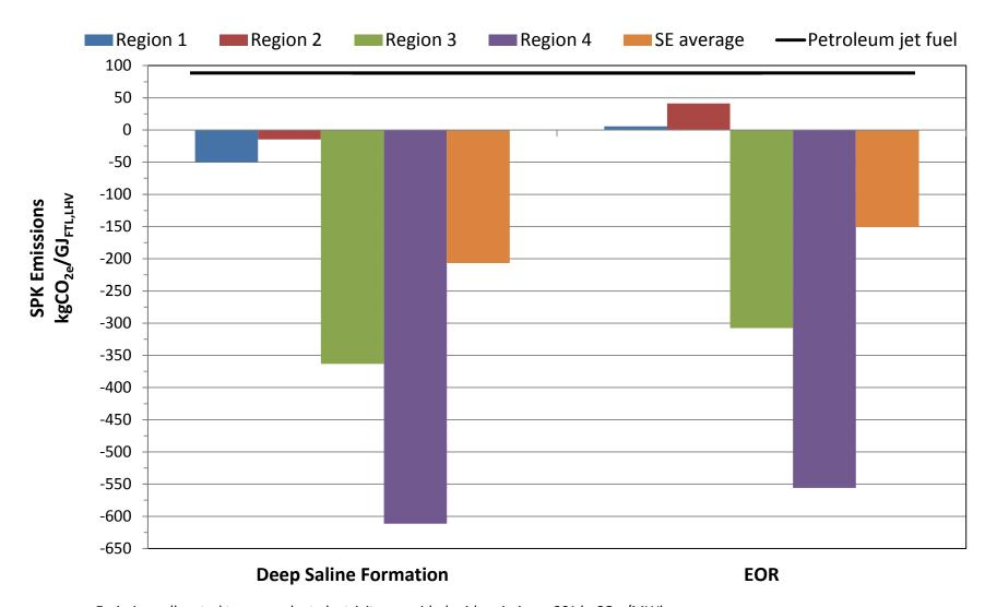
Emissions allocated to co-product electricity = avoided grid emissions:  $661 \text{ kgCO}_{2e}/\text{MWh}$ . Emissions allocated to co-product naphtha represented by avoided emissions from petroleum-derived gasoline:  $91.4 \text{ kgCO}_{2e}/\text{GJ}_{1HV}$ .
