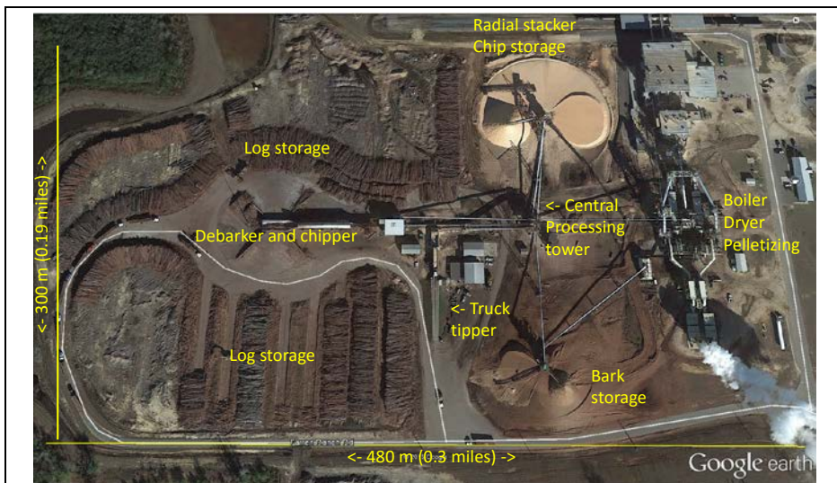
Figure 5. Example of log storage and preparation system similar to that for the LBJ plant (Green Circle Bioenergy in Florida), except that the LBJ facility will not include the “Boiler/Dryer/Pelletizing”) and will process about one-fifth as much biomass as this facility.
