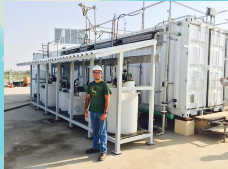
System in operation, producing WHO quality water at <1.0\text{kWh}/\text{m}^3 .
