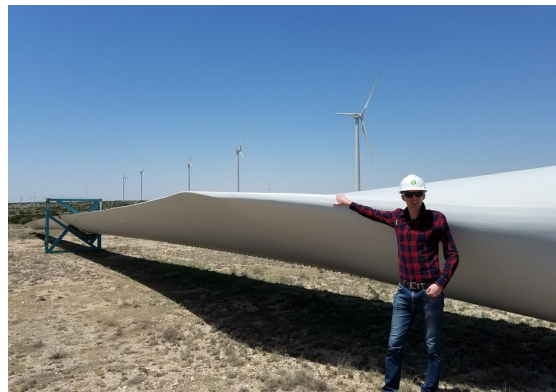
Figure 5.2: A 50-meter blade stored at ground level, being examined by one of the authors (Greg Davies) at the Sherbino 2 wind farm in western Texas. The blade is viewed from its root, looking toward its tip; it is thicker at its base, twisted, and tapered. Photo: Ryan Edwards.
