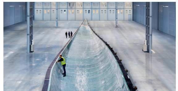
Figure 5.7: Top: Looking inside a turbine blade (the BP Sherbino Mesa II turbine blade) at its two shear webs and its balsa/fiberglass construction. Photo: Greg Davies. Bottom: A facility for the fabrication of turbine blades, showing the mold for a half-blade. Photo: Siemens AG, Munich/Berlin, https://www.siemens.com/press/en/presspicture/?press=/en/presspicture/pictures-photonews/2012/pn201204.php .
