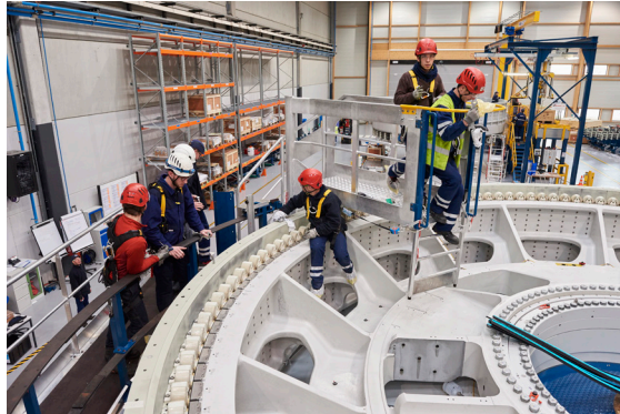
Figure 6.5: The manufacture of a permanent magnet generator. The permanent magnets are the silver brick-shaped objects, arrayed end-to-end along the inner perimeter of the stator; the left hand of the operator standing inside the stator is nearly touching one. Photo: General Electric, https://www.ge.com/reports/where-ge-makes-haliade-turbines/ .
